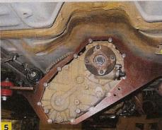
Frame and axle brackets are all laser-cut and fully welded and come with all necessary hardware. This is the "basic" kit from Off Road Solutions. Considering the multitude of parts, it doesn't look very basic to us! However, this kit can be installed by a competent do-it-yourselfer.
